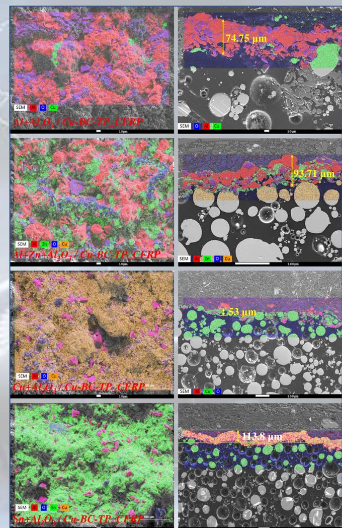
Fig. 3 Results of mixed powders cold sprayed on the substrates of Cu-BC-TP\_CFRP
