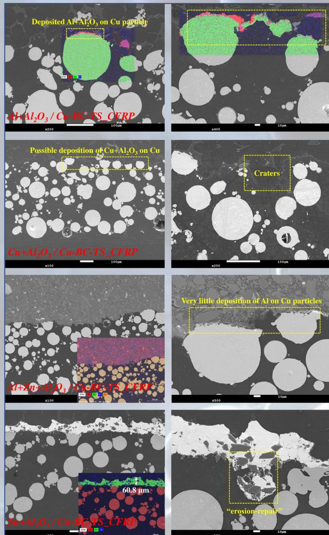
Fig. 1 Results of mixed powders cold sprayed on the substrates of Cu-BC-TS\_CFRP
